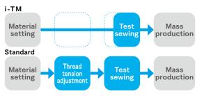
As the appropriate thread tension adjustment is applied regardless of the thread type, mass production can be started quickly.
