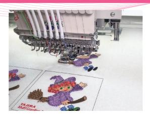
The cutting device can be equipped on TMCR-VF series. As the cord can be automatically cut at the timing of color change, the productivity of multi-colored code embroidery is drastically improved.
